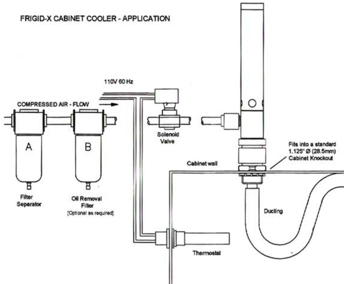
Filtered, compressed air enters the Nex Flow™ Frigid-X™ Electrical Panel Cabinet Cooling System Air Conditioner and through the vortex tube component. The air is split into into two streams, one hot and one cold.
